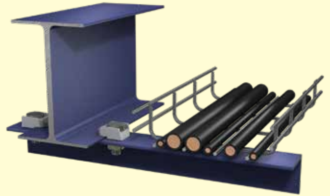
Cantilevered angle support for running cable tray
