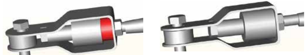
Figure 20 - Un-tensioned Tension Indicator Figure 21 - Correctly tensioned Tension Indicator
