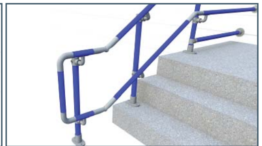
F) EXTENSIONS: Stairs: Handrails should extend the width of one stair tread and then level out for 300mm Ramps: Handrail should extend parallel to walking surface 300mm past the top and bottom of the ramp.
