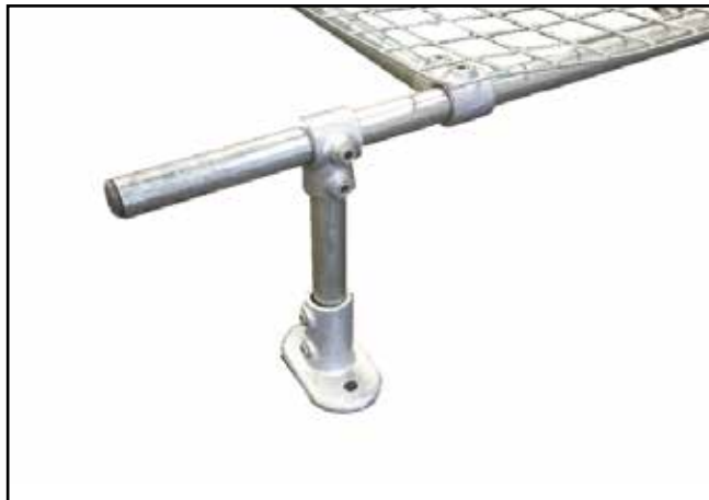
J. Slide 1 No. Rail Flange fitting over each end of the exposed tube in the corners of the frame. Carefully align the fitting to ensure it is positioned on the crown of roof sheet.
