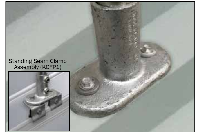
K. Carefully cut 6No. 120mm lengths of sealing strip. Place the Sealing Strip between the 6No. Standard Rail Flange fittings and the roof structure. Use Self Drilling Screws (SDS55X550) to attach the screen onto the roofing sheet. NB If attaching to standing seam roof use KCFP1 clamps to connect to the standing seam and bolt the 62-5 fitting to the KCFP1 clamp as shown in the diagram.
