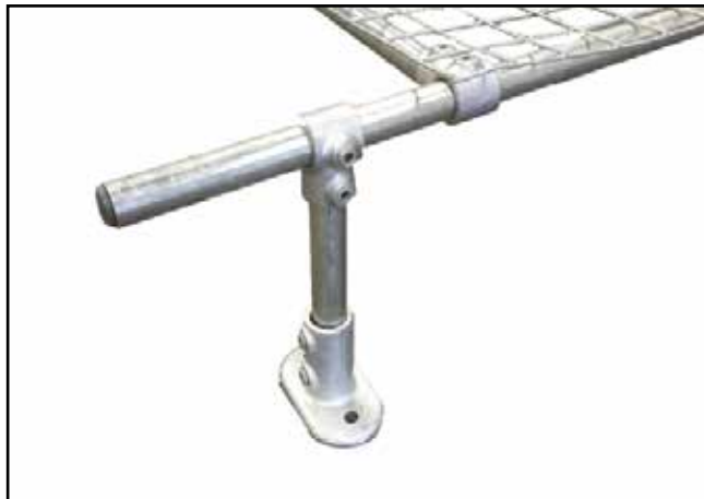
J. Assemble 6No. legs as above diagram using a (62-5) Standard Rail Flange fitting and a (10-5) Single Socket Tee fittings and 200mm tube. Line up with crowns of roofing material and tighten to 39Nm.
