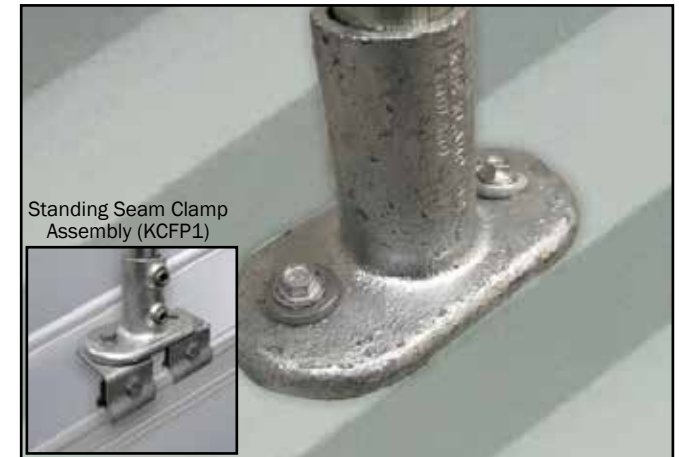
K. Carefully cut 6No. 120mm lengths of sealing strip. Place the Sealing Strip between the 6No. Standard Rail Flange fittings and the roof structure. Use Self Drilling Screws (SDS55X550) to attach the screen onto the roofing sheet. NB If attaching to standing seam roof use KCFP1 clamps to connect to the standing seam and bolt the 62-5 fitting to the KCFP1 clamp as shown in the diagram.
