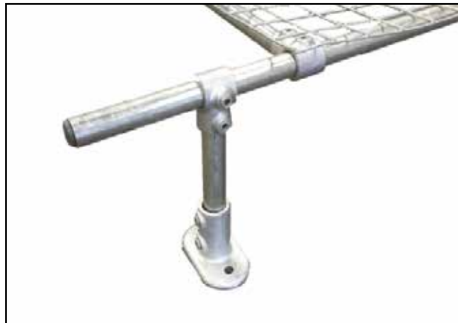
J. Assemble 4No. legs as above diagram using (62-5) Standard Rail Flange fitting and (10-5) Single Socket Tee fittings and 200mm tubes. Line up with crowns of roofing material and tighten to 39Nm.
