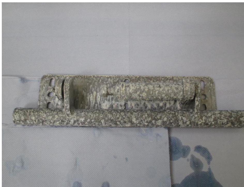
Fig 2: Photograph showing the condition of the Sample after 72 hours Salt Spray Test
