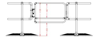
The distance between the bottom rail and the flooring must be less than 500mm. There are two ways to achieve this: use a full height gate, which fills that void or use our KEE GATE, which features a large D bend to meet these requirements.
