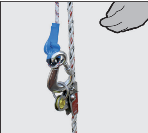
k. Position the Rescue Kernmantel Rope over the Edge Protector. Now carefully lower the Rescue Rope Grab down towards the casualty. The Rescue Rope Grab device will descend easily under gravity to the “D” ring of the casualty’s harness.
