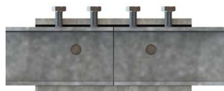
Correct alignment - Side view
