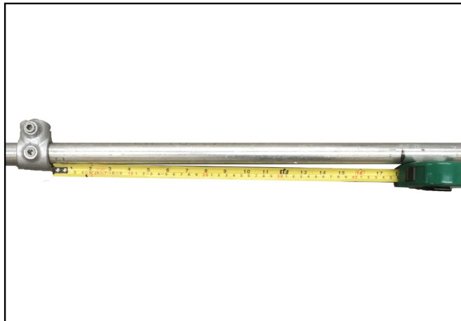
C. Carefully measure 455mm from each side of the centre point and mark. Slide a (10-5) Single Socket Tee to align with each of the four marked positions, rotate fitting to ensure correct orientation (see stage E) and tighten the grub screws using a 1/4" Allen Key. NB If further extension panels are to be used then replace 2no. (10-5) Single Socket Tee for 2No. (26-5) Two Socket Cross fittings as this will permit further panels to be linked.
