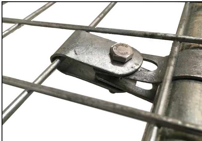
I. Mesh panel clips are to be attached as above, 2 squares in from the edge of the mesh panel.
