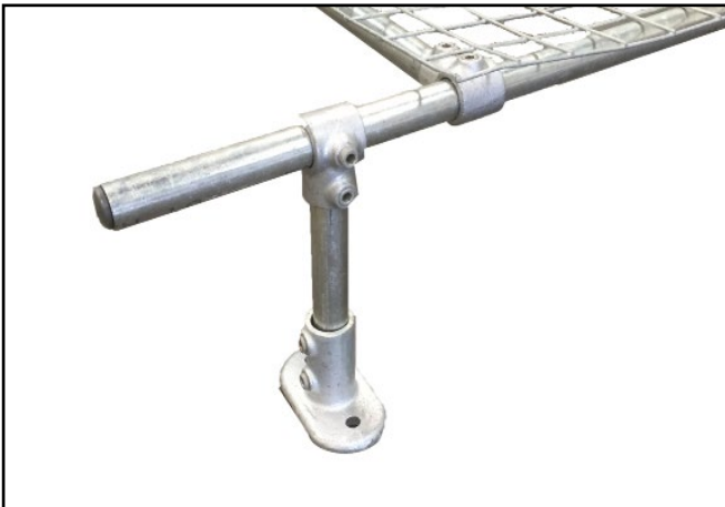
J. Assemble 2No. legs as above diagram using (62-5) Standard Rail Flange fitting and (10-5) Single Socket Tee fittings and 200mm tubes. Line up with crowns of roofing material and tighten to 39Nm.
