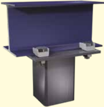
Column end plate to I-Section
