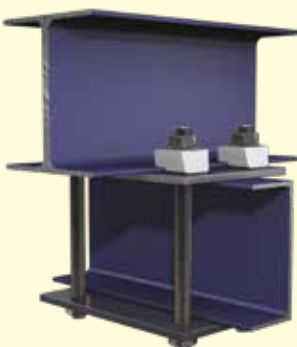
Channel section below I-Section at 90 degrees
