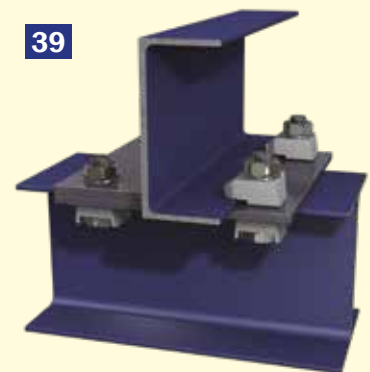
Channel positioned above I-Section at 90 degrees
