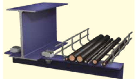
Cantilevered angle support to I-Section
