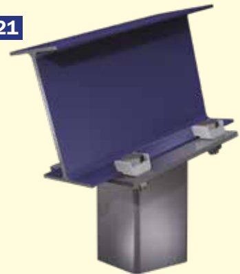
Column end plate to sloping I-Section
