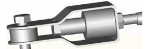
Figure 21 - Correctly tensioned Tension Indicator
