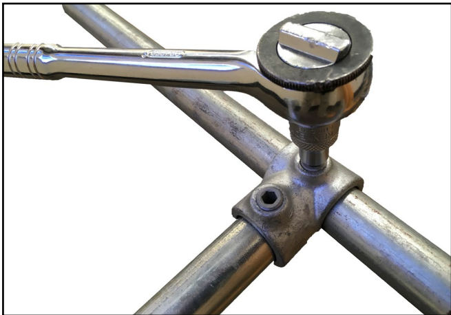
F. Using a 1/4" Allen Key ensure all grub screws are finally tightened.
