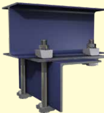
Angle section below an I-Section at 90 degrees
