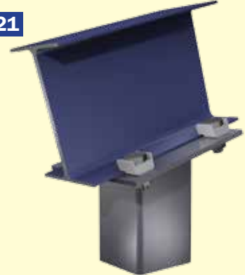
Column end plate to sloping I-Section
