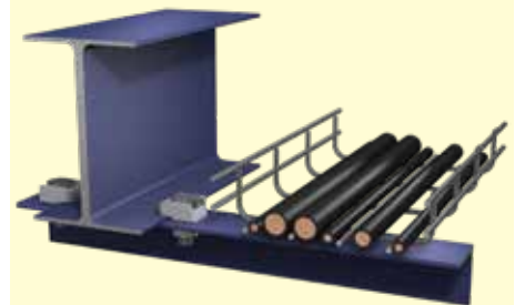
Cantilevered angle support to I-Section
