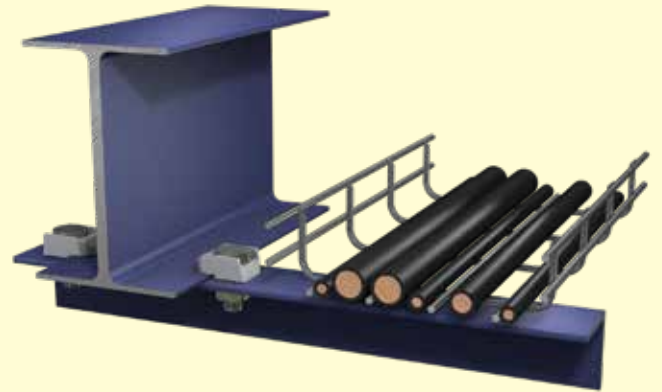
Cantilevered angle support for running cable tray
