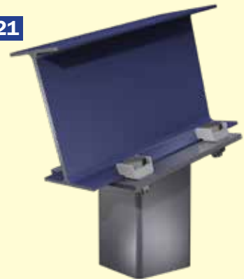
Column end plate to sloping I-Section
