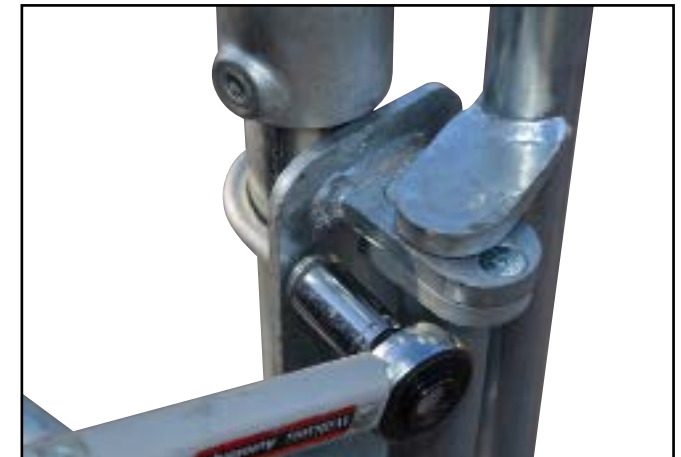
E. Torque all nuts/U Bolts to 25Nm using the 13mm or 17mm socket and torque wrench.
