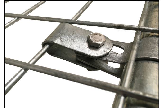
I. Mesh panels clips are to be attached as diagram above, 2 squares in from the edge of the mesh panel.
