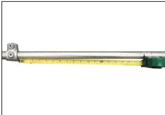
C. Measure 995mm from the centre point of each of the 3000mm tubes and slide a (10-5) Single Socket Tee into each of the four marked position and tighten the grub screws using a 3/16" Allen Key. NB If further extension panels are to be used then replace 2no. (10-5) Single Socket Tee for 2No. (26-5) Two Socket Cross fittings this will permit further panels to be connected to the primary.
