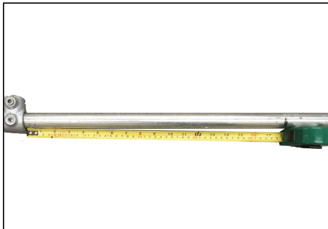
C. Carefully measure 455mm from each side of the centre point and mark. Slide a (10-5) Single Socket Tee to align with each of the four marked position, rotate fitting to ensure correct orientation (see stage E) and tighten the grub screws using a 1/4" Allen Key. NB If further extension panels are to be used then replace 2no. (10-5) Single Socket Tee for 2No. (26-5) Two Socket Cross fittings as this will permit further panels to be linked.
